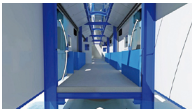
Central aisle with ventilation distribution to the rooms.
