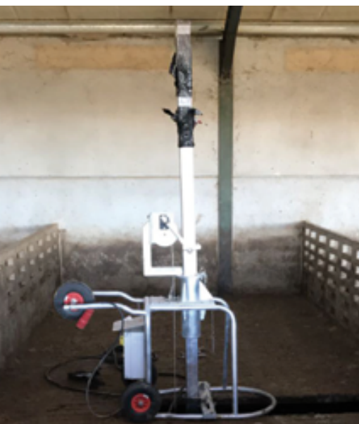
MIXER IN INTERIOR PIT
